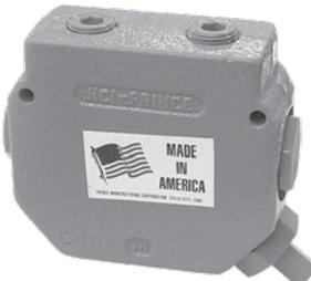
The PRINCE model RD-500P is a pressure compensated proportional flow divider valve with one fixed and one adjustable orifice. This valve provides the same function as the RD-200 except the divider ratio can be changed in the field.
