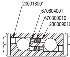
The RD-300AB valve has a built-in automatic bypass. This allows oil to crossover from one outlet to the other when the pressure difference between the two outlet reaches 750 PSI.
