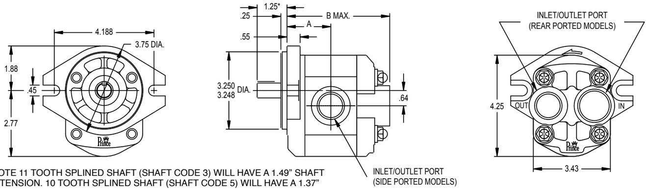
\*NOTE 11 TOOTH SPLINED SHAFT (SHAFT CODE 3) WILL HAVE A 1.49" SHAFT EXTENSION. 10 TOOTH SPLINED SHAFT (SHAFT CODE 5) WILL HAVE A 1.37" SHAFT EXTENSION.
