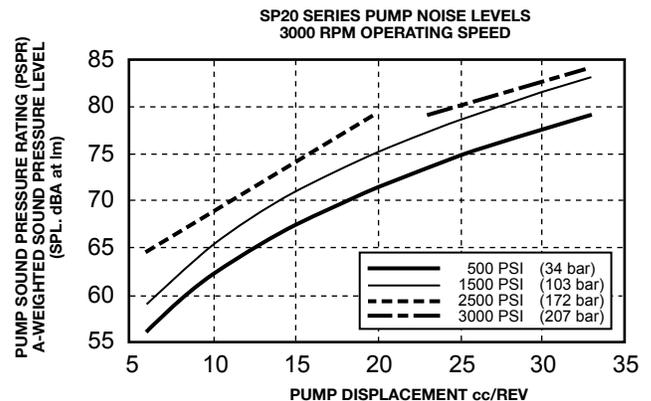
Pump acoustical data was determined in accordance with ANSI/B93.71M. Hydraulic fluid power-Pumps-Test code for the determination of airborne noise levels
